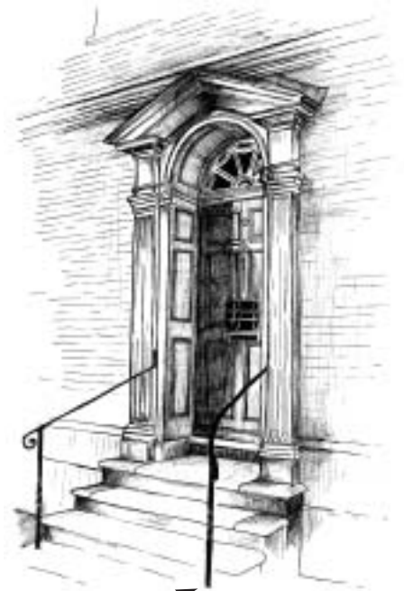
Simple handrails do visually better than modern over-decorative replicas of late Victorian castings.
